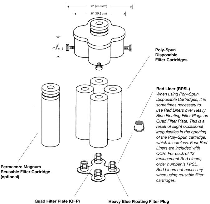
Insert Blue Filter Plugs through holes in polypropylene plate.
